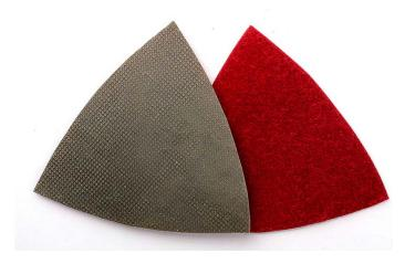
The triangular polishing pads are used for FEIN MultiMaster type oscillation tools for detailed polishing of granite, marble, concrete and other types of stones. They are 3" for each side. The entire set comes with grite 60# 120# 200# 400#. they can be used for wet. the triangle diamond polishing pads are also suitable for Dremel Multi-Max, Rockwell SoniCrafter, as well as Ryobi detail.
