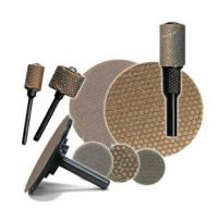
Flexible Diamond bands and discs are made from a two-ply polyester backing film evenly coated with diamond filled nickel plated dots. These flexible diamond bands have been designed and developed for light grinding, shaping and polishing applications with contours and hard to
