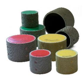
M14 fitting, flexible diamond vanity drums with central water feed for wet grinding and polishing internal cutouts in glass. The diamond vanity drums are color coded M60 green, M120 black, M200 red and M400 yellow for easy grade identification.
